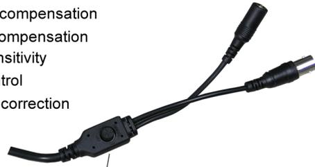
The 3-dimensional mini-joystick on the video/power cable gives the user quick access to the OSD menu. Move it left/right, up/down and "click" to navigate the menu and make selections.
