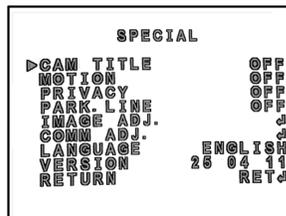
Most common camera adjustments are easy to find in the on-screen menu. Special functions, like privacy masking and motion detection, are also built into the chipset making this camera adaptable for many surveillance environments.
