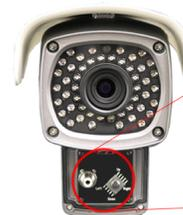
RCA Connector for Video Test monitor
