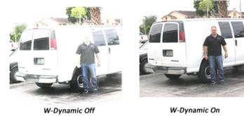
W-Dynamic enhances the image so that subjects in the foreground or in a shadow are not washed-out by an object with high brightness nearby, even with rapid changes in the light source position, direction or intensity. W-Dynamic reacts faster and more accurately than standard dynamic range.
